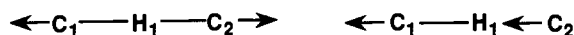
Figure 3. Schematic representation of the normal modes A 1g (left) and A 2u (right) of TS(A).
